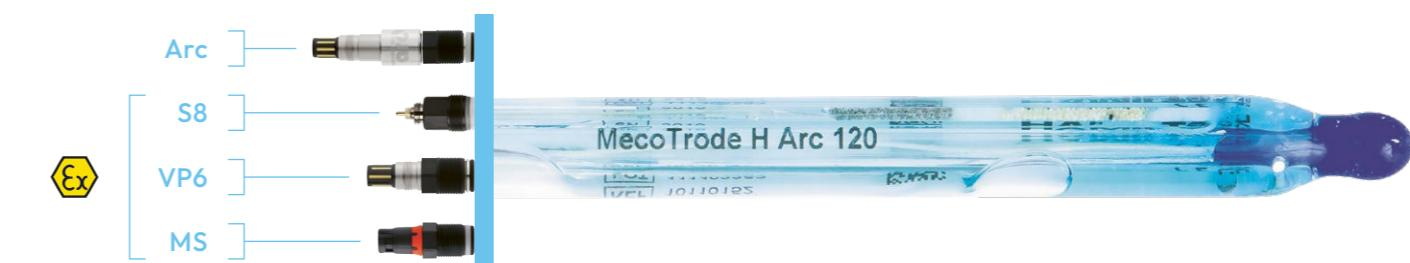
The MecoTrode pH sensors are designed for processes in the chemical industry with extreme pH values. They are constructed from a H-glass type membrane which provides a low alkaline error and stable measurement even at high temperatures. Three high-performance ceramic diaphragms reduce the effect of flow potential in viscous liquids.
