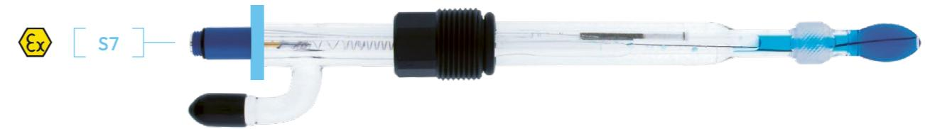
The IonoTrode sensor is designed for applications in ion-weak media and high purity water measurements. The F glass membrane has a very low resistance, therefore the sensor can be used in samples with low conductivity, where it offers the highest accuracy over a long period of time. There is a storage container with 3 M KCl attached via a tube to the side-arm of the IonoTrode and the flow-out of the electrolyte can be controlled with the sleeve diaphragm.
