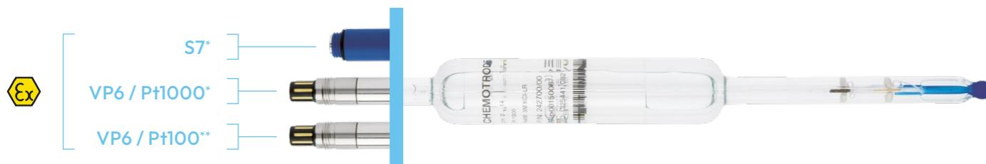
This is our most robust sensor, designed for measuring pH in demanding applications in pharmaceutical and chemical industries. The Everef-F reference cartridge ensures that the reference electrolyte remains free of silver and precipitation, while the liquid electrolyte can be easily refilled and pressurized up to 6 bar through a port in the sensor for easy maintenance. Refillable liquid electrolyte ensures fast response times and high precision during measurements.
